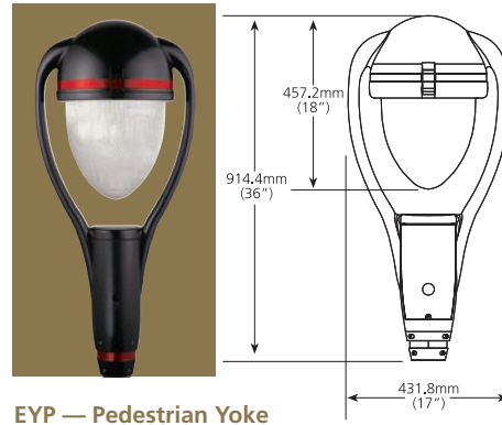
EYP — Pedestrian Yoke Maximum Weight: 19 kg. (42 lbs.) Maximum EPA: 1.08
